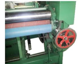
Bearing embedded continuous take-up mechanism
